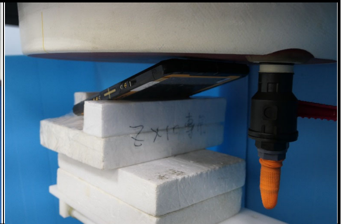
Right Curve 1 of Tablet Mode Tested at 0 mm
