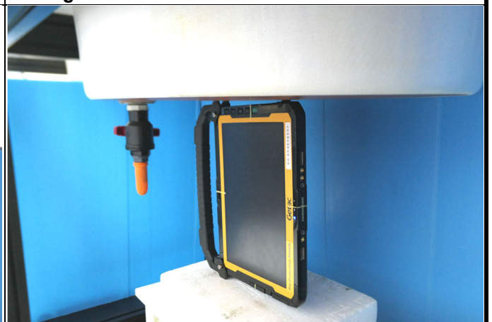
Right Side with Handle of Tablet Mode Tested at 0 mm
