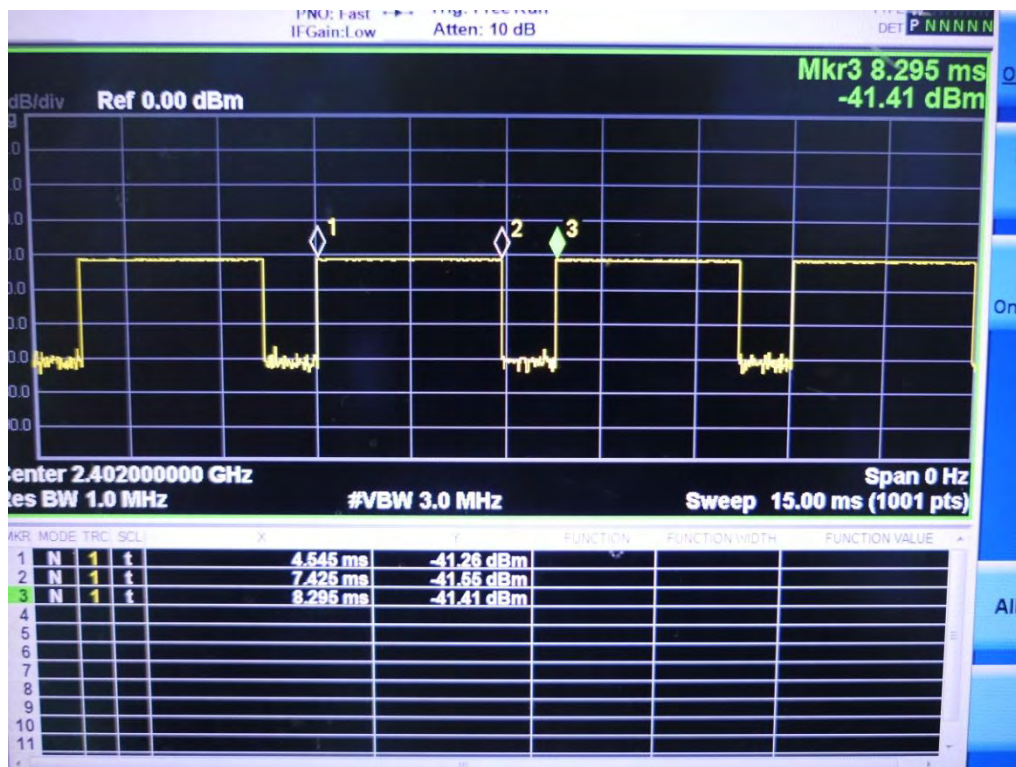
Time-domain plot for Bluetooth transmission signal
