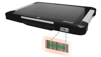
**NOTE:** If the code being scanned is highly reflective (e.g., laminated), it may be necessary to tilt the code +5° to prevent unwanted reflection.
