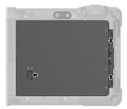
1. Slide the three battery latches to the unlocked position (  $\bigcirc$  ).
