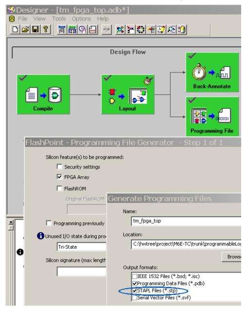
2. Generate the DAT file - Once the \*.stp file has been generated it can be fed into the datgen.exe utility to generate the .dat file. datgen must be run from the command line.
