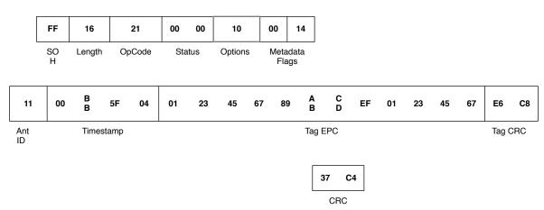
Here is another example request and response showing the use of <u>Tag Singulation/Select</u> <u>Functionality</u> and getting the tag metadata for the specified tag:
