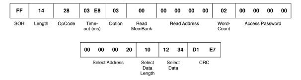
If Option=0x00 or 0x01 is used then the unused <u>Tag Singulation Fields</u> (including the Access Password) must be removed from the request.
