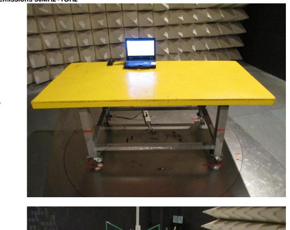
For radiated emissions 30MHz~1GHz
