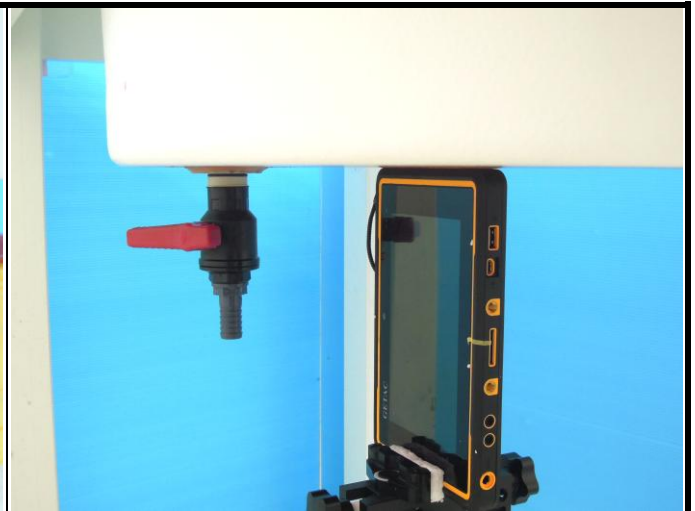
Right Side of EUT with 0 cm Gap
