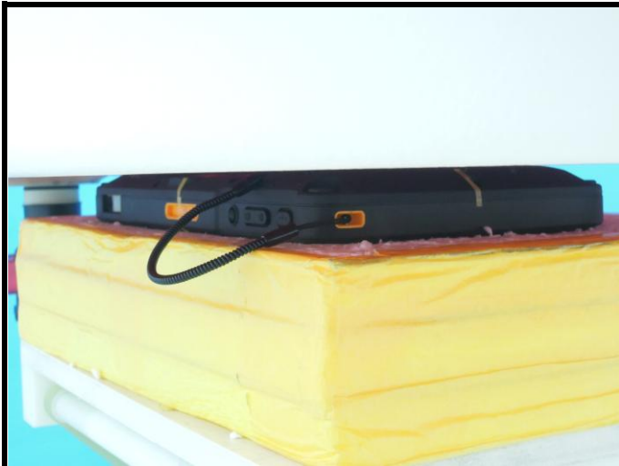
Rear Face of EUT with 0 cm Gap
