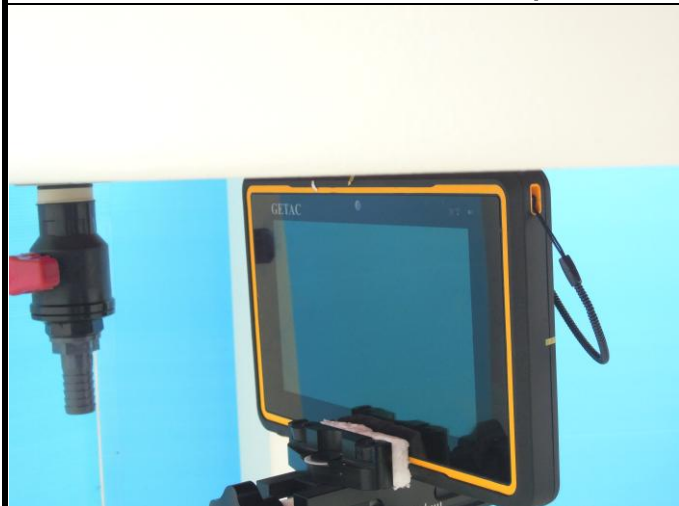
Top Side of EUT with 0 cm Gap
