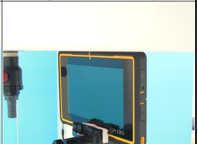
Bottom Side of EUT with 0 cm Gap
