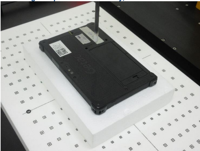
Testing Setup for Power Density, Rear Face at 0 mm
