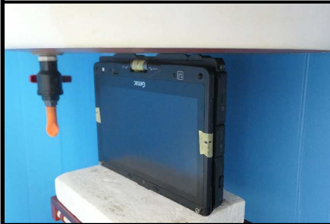
Bottom Side of EUT Tested at 0 mm
