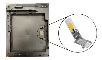
3. Close the holder tray and slide it back to the locked position.
