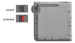
**CAUTION:** Make sure the lock is correctly locked, not revealing the underneath red part.
