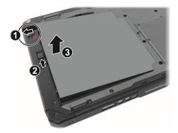
3. Fit another battery pack into place. With the battery pack correctly oriented, attach its connector side to the battery compartment at an angle (●) and then press down the other side (●). The battery release latch should automatically engage.
