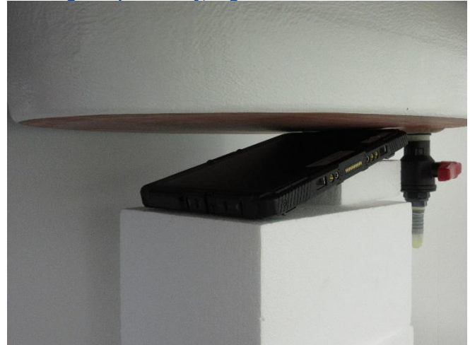
Testing Setup for Body, Right Side of Antenna at 0 mm
