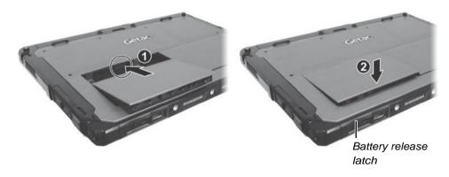
2. Slide the lock of the battery release latch downward to the locked position.
