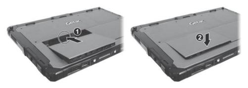
5. Slide the lock of the battery release latch downward to the locked position.
