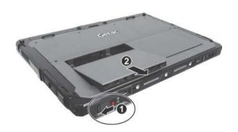
4. Fit another battery pack into place. With the battery pack correctly oriented, attach its connector side to the battery compartment at an angle () and then press down the other side (). The battery release
