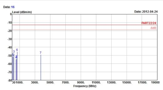
Site : 966 Chamber 5 Condition : PART22/24 3m EIRP\_RSE\_1G~19G\_3 VERTICAL
