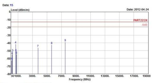
Site : 966 Chamber 5 Condition : PART22/24 3m EIRP\_RSE\_1G~19G\_3 HORIZONTAL
