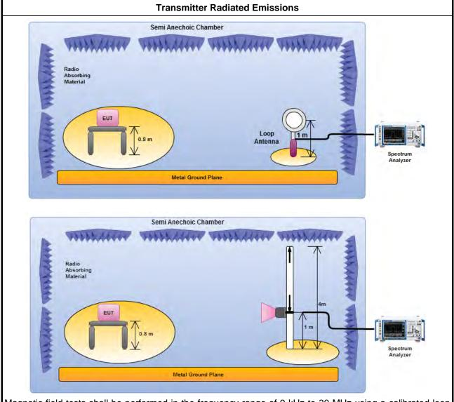
Magnetic field tests shall be performed in the frequency range of 9 kHz to 30 MHz using a calibrated loop antenna. The center of the loop shall be 1 m above the ground. Electric field tests shall be performed in the frequency range of 30 MHz to 1000 MHz using a calibrated bi-log antenna. the antenna height shall be varied from 1 m to 4 m.
