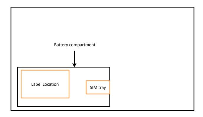
Label located in the battery compartment and is visible to the users as they install the SIM card.
