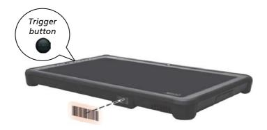
**NOTE:** If the code being scanned is highly reflective (e.g., laminated), it may be necessary to tilt the code +5° to prevent unwanted reflection.
