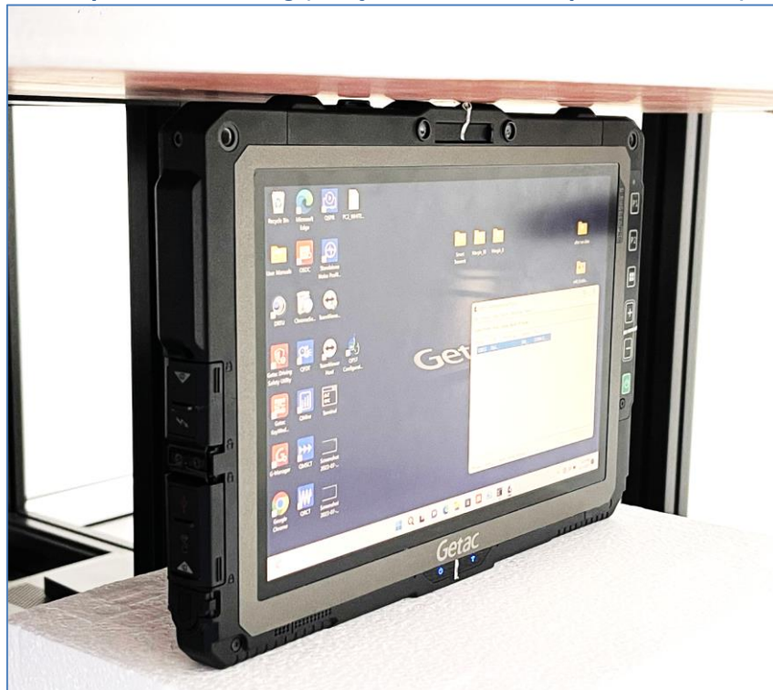
Setup for SAR Testing (Body, Tablet mode, Top Side at 0 mm)
