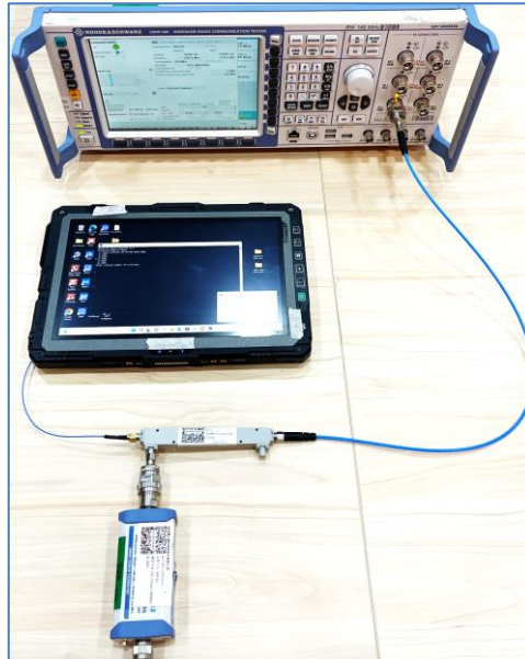
Setup for Conducted Power Testing (Figure 4-4)
