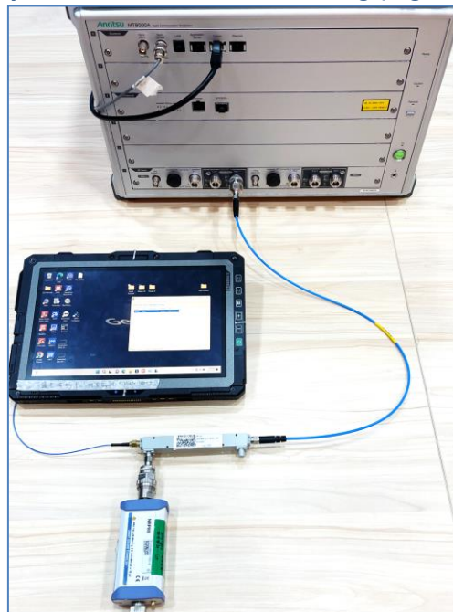
Setup for Conducted Power Testing (Figure 4-4)
