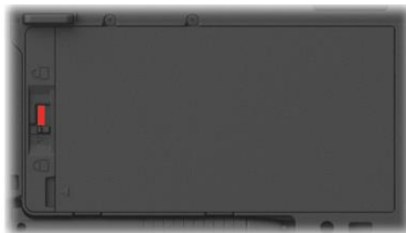
Incorrect (revealing red part)
