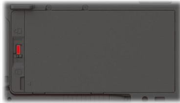
Incorrect (revealing red part)
