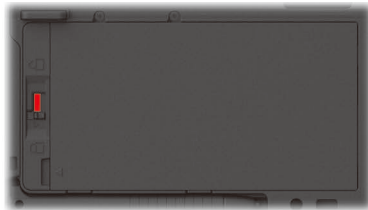
Incorrect (revealing red part)
