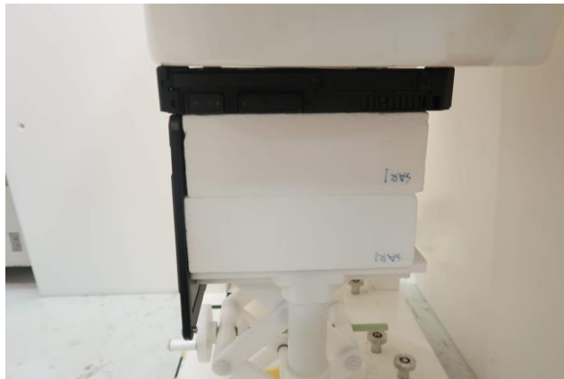
Bottom of Laptop, Test Separation 0 mm _ SKUA
