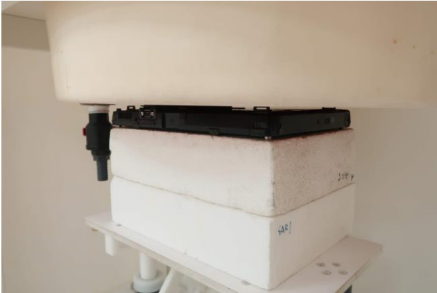
Bottom Face, Test Separation 0 mm
