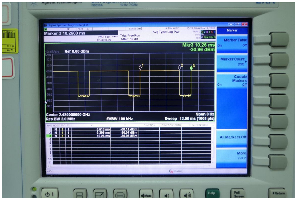
Time-domain plot for Bluetooth transmission signal
