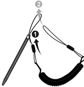
2. Insert the other loop end to the tether hole on the Tablet PC (as indicated by ❶ below). Then, insert the stylus end through the loop (as indicated by ❷ below) and pull it tight.
