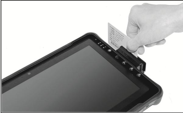
**NOTE:** Make sure to press the magnetic stripe firmly against the reader when swiping the card. A poor contact or an incomplete swipe action will result in an unsuccessful reading.
