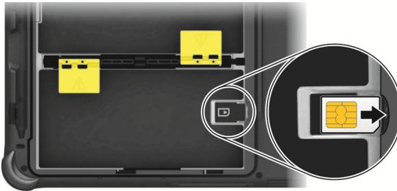
**NOTE:** To remove the SIM card, just push in the SIM card to pop-out and remove the card.
