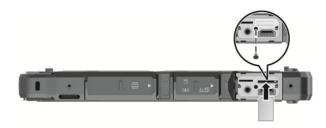
NOTE: To remove the micro-SIM card, just push in the card to release it and then pull it out.
