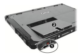
4. Fit another battery pack into place. With the battery pack correctly oriented, attach its connector side to the battery compartment at an angle ( ) and then press down the other side ( ). The battery latch should automatically engage.
