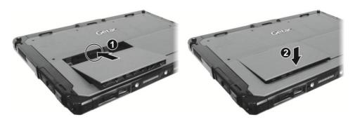
3. Slide the lock of the battery latch downward to the locked position.
