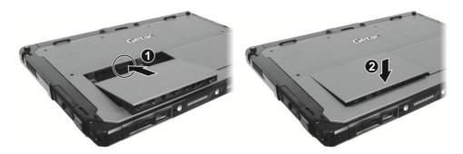
5. Slide the lock of the battery latch downward to the locked position.
