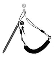
2. Insert the other loop end to the tether hole on the Tablet PC (as indicated by ① below). Then, insert the stylus end through the loop (as indicated by ② below) and pull it tight.
