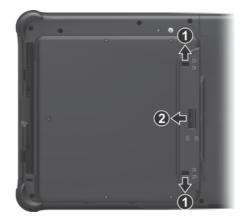
2. Pull the ribbon strip to lift the battery pack off the compartment.
