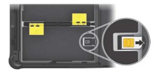
**NOTE:** To remove the SIM card, just push in the SIM card to pop-out and remove the card.
