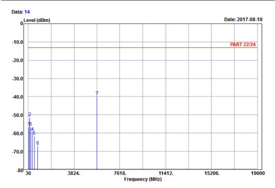
Site : 966 chamber 1 Condition: PART 22/24 Vertical Remark : Band II\_Link\_CH9538
