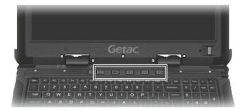
The Quick Buttons allow you to quickly start a program or activate a function. Default functions are:
