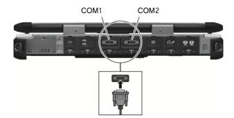
**NOTE:** The serial port is configured as RS232 by default. If you want to use it as RS422, run BIOS Setup to change the setting. (See "Advanced Menu" in Chapter 5 for information.)
