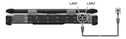
Your computer supports two LAN modules (LAN1 and LAN2) so you can connect to two networks at the same time.
