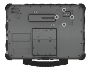
4. Locate the SIM card slot. Locate the SIM card slot. Slide the locking tab inward to unlock (①). Lift the slot up and, noting the orientation, insert the SIM card into the slot (②). Slide the locking tab outward to secure the SIM card in place (③).
