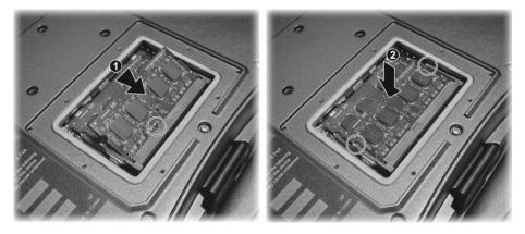
**CAUTION:** If the RAM module is difficult to insert or difficult to push down, do not force it. Check once more to ensure that the module is positioned correctly.
