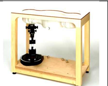
Fig 5.8 Photo of SAM Phantom
