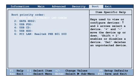
The bootable devices will be automatically detected during POST and shown here, allowing you to set the sequence that the BIOS uses to look for a device from which to load the OS. See the information on the right side of the menu for keyboard usage.
