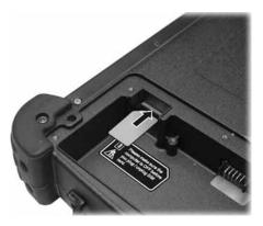
To remove the SIM card, just push in the SIM card to pop-out and remove the card.
