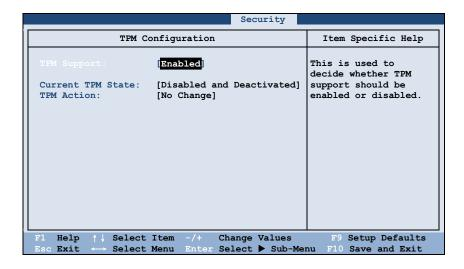
**TPM Support** enables or disables TPM (Trusted Platform Module) support. TPM (Trusted Platform Module) is a component on your computer's mainboard that is specifically designed to enhance platform security by providing a protected space for key operations and other security critical tasks.
