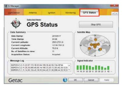
To start GPS positioning, click **Start GPS**. The screen displays:
