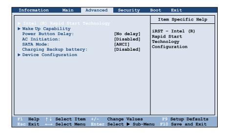
Intel (R) Rapid Start Technology cofigures iRST. Press Enter to access the submenu as shown below.
