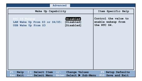
RTC S4 Wakeup enables or disables the RTC (Real Time Clock) wakeup from S4 (Hibernation) feature when AC power is connected. Set this item to Enabled if you use Windows task scheduler to have the computer automatically perform tasks at specific times.
