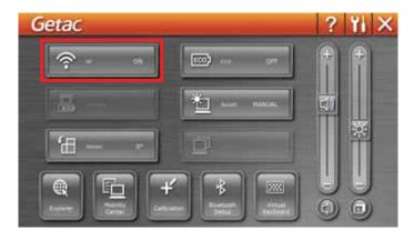
3. Windows Mobility Center has wireless network turned on by default. The Wireless Network icon and on the taskbar should appear without a red X. (In case you have previously turned it off in Windows Mobility Center, be sure to turn it on when using the function the next time.)
