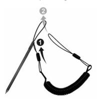
2. Insert the other loop end to the tether hole on the Tablet PC (as indicated by ● below). Then, insert the stylus end through the loop (as indicated by ● below) and pull it tight.
