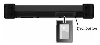
3. When a new card is seated, the Tablet PC will detect it and try to install the appropriate driver. Follow the on-screen instructions to complete the process.
