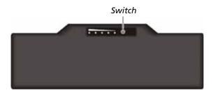
The value of the corresponding green segment indicates the relative percentage of the battery charge. The battery pack is fully discharged when you see no segment glowing green.
