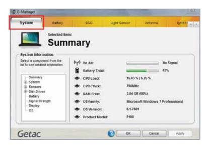
To view specific information, select the component from the list on the left side of the screen. The information of the selected component will be displayed on the right side of the screen.
