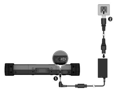
7. Power is being supplied from the electrical outlet to the AC adapter and onto your Tablet PC. Now, you are ready to turn on the Tablet PC.
