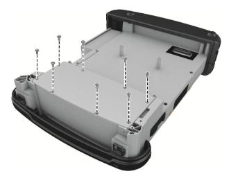
5. Fit the battery pack into place (**0**). Tighten two screws (**0**).
