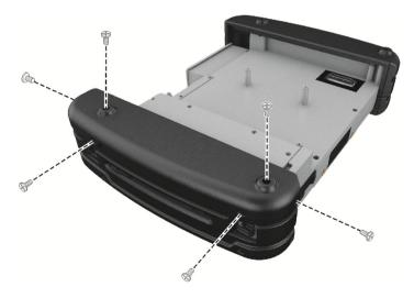
4. Remove the battery cover by unfastening 8 screws (as shown below) from the cover.
