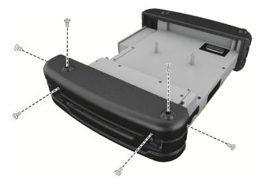
3. Remove the battery cover by unfastening 8 screws (as shown below) from the cover.
