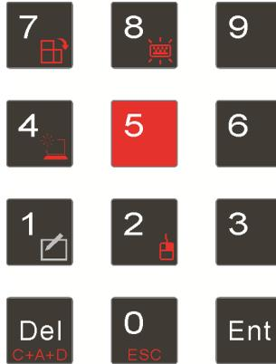
When the **Fn** keylock is ON (indicated by the icon
