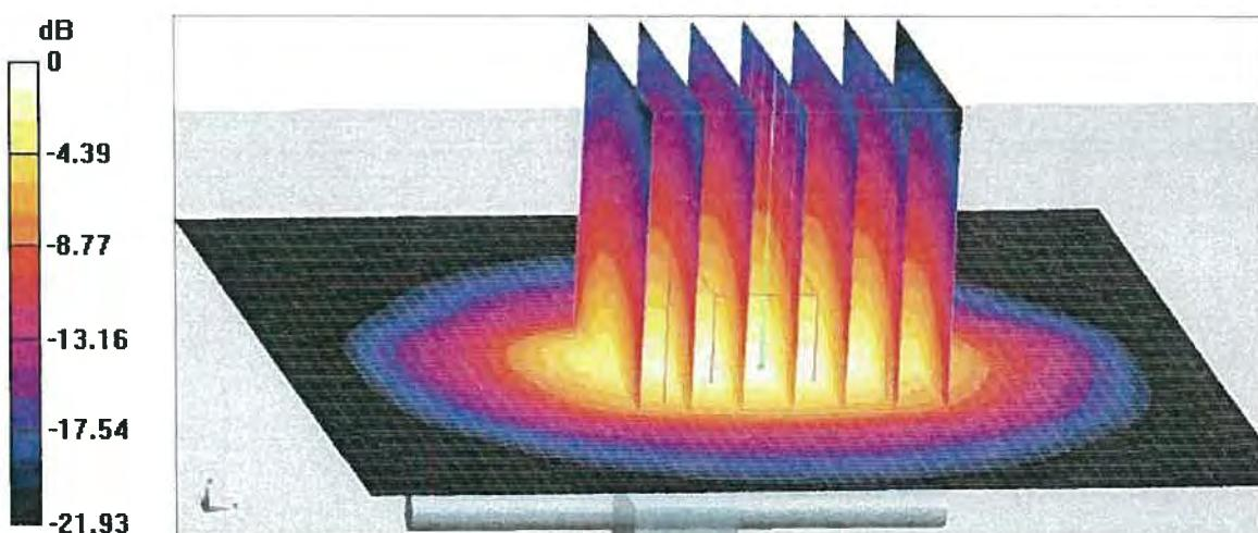
$$0 \text{ dB} = 21.9 \text{ W/kg} = 13.40 \text{ dBW/kg}$$
