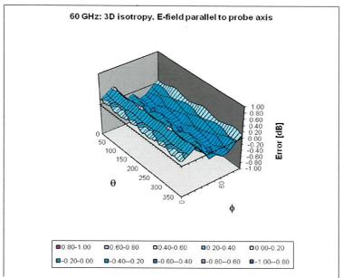
Probe isotropy for  $E_{tot}$ : probe rotated  $\phi$  = 0° to 360°, tilted from field propagation direction  $\overline{k}$  Parallel to the field propagation ( $\psi$  =0° - 90°) at 30 GHz: deviation within ± 0.42 dB Parallel to the field propagation ( $\psi$  =0° - 90°) at 60 GHz: deviation within ± 0.46 dB
