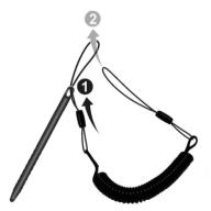
Insert the other loop end to the tether hole on the Tablet PC (as indicated by
