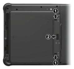
2. Note the orientation of the battery pack. Hold the battery pack at an angle and insert its small tabs to the corresponding notches in the battery compartment. Then, lift the yellow protection sheet in the battery compartment and plug the battery connector.
