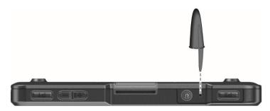
Alternatively, you can force the device to power off by pressing and holding the power button for more than 10 seconds. Then turn it on again.
