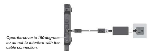
2. Power is being supplied from the external power source to MX50.
