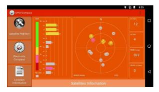
SBAS (satellite-based augmentation system) provides additional accuracy and reliability for the GPS devices. Ground stations are necessary to achieve the purpose. The SBAS feature works where such stations exist. You can enable the SBAS feature. (See "Getac Settings" in Chapter 6.)
