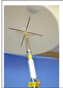
Construction: Symmetrical dipole with I/4 balun Enables measurement
