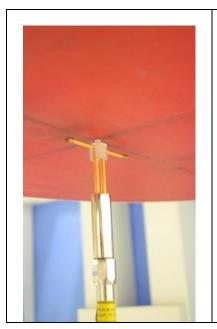
**Construction:** Symmetrical dipole with I/4 balun Enables measurement of
