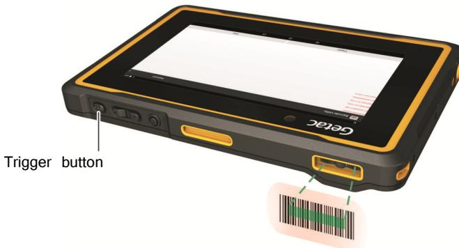
**NOTE:** Improper ambient light and scanning angle can affect the scanning results.
