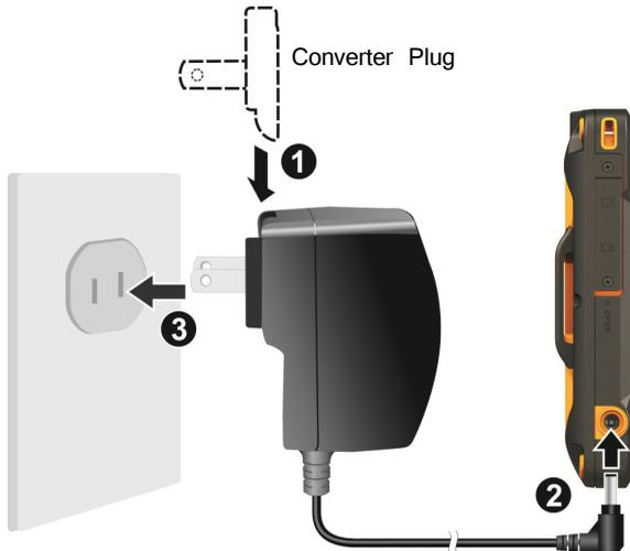
3. The charge indicator glows in amber when charging is in progress. Do not disconnect your device from AC power until the battery is fully charged, as indicated by the amber indicator turning into green. This will take a couple of hours.
