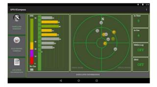
SBAS (satellite-based augmentation system) provides additional accuracy and reliability for the GPS devices. Ground stations are necessary to achieve the purpose. The SBAS feature works where such stations exist. You can enable the SBAS feature. (See "Getac Settings" in Chapter 7.)
