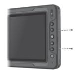
2. Noting the orientation, insert the SIM card all the way into the slot.
