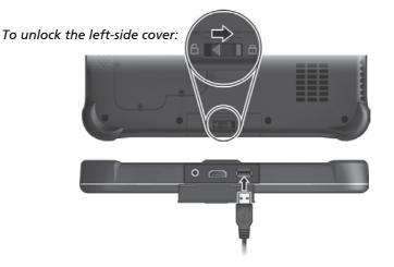
Select models have a second USB port, which supports USB 2.0 (transfer rate is 480 MB/s).
