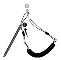
Insert the other loop end to the tether hole on the Tablet PC (as indicated by ● below). Then, insert the stylus end through the loop (as indicated by ● below) and pull it tight.
