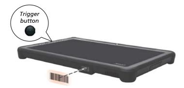
**NOTE:** If the code being scanned is highly reflective (e.g., laminated), it may be necessary to tilt the code +5° to prevent unwanted reflection.
