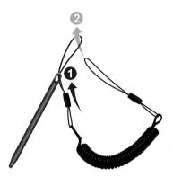
2. Insert the other loop end to the tether hole on the Tablet PC (as indicated by **1** below). Then, insert the stylus end through the loop (as indicated by **2** below) and pull it tight.
