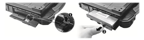
**NOTE:** The position of the release latch and ribbon strip varies with the device. Only one example is shown here.
