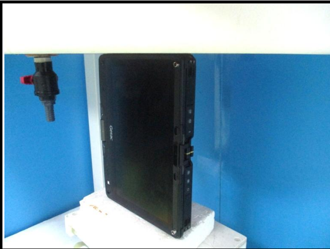
Left Side of EUT with 0 mm Gap (Tablet PC Mode)
