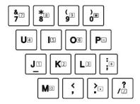
Numeric keys facilitate entering of numbers and calculations. When Num Lock is on, the numeric keys are activated; meaning you can use these keys to enter numerals.
