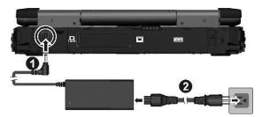
3. Power is being supplied from the electrical outlet to the AC adapter and onto your computer. Now, you are ready to turn on the computer.
