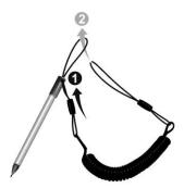
2. Insert the other loop end to the hook on the computer (as indicated by **1** below). Then, insert the stylus end through the loop (as indicated by **2** below) and pull it tight.
