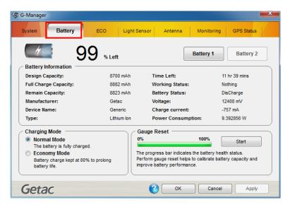
The battery items shown in the screen depend on your computer model. You may see up to two battery items (**Battery 1** and **Battery 2**). Click a battery item to view the information of the selected battery. Batteries not installed in your computer are grayed-out.
