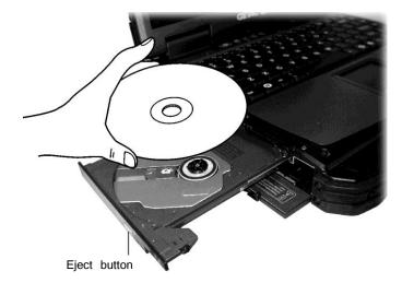
To remove a disc, hold the disc by its outer edge and lift it up from the tray.
