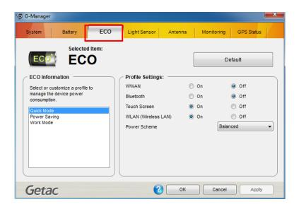
To put the system into an ECO mode, use the **ECO** button. (See "Using the Quick Buttons" in Chapter 2 for information.)
