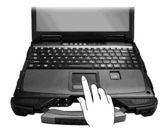
The touchpad consists of a rectangular pad (work surface) and a left and right buttons. To use the touchpad, place your forefinger or thumb on the pad. The rectangular pad acts like a miniature duplicate of your display. As you slide your fingertip across the pad, the pointer (also called cursor) on the screen moves accordingly. When your finger reaches the edge of the pad, simply relocate yourself by lifting the finger and placing it on the other side of the pad.
