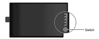
The value of the corresponding green segment indicates the relative percentage of the battery charge. The battery pack is fully discharged when you see no segment glowing green
