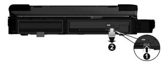
4. With the ribbon strip facing outward, insert the new device all the way into the media bay.
