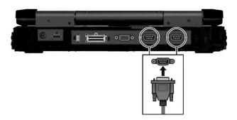
NOTE: Portable modems that derive power through the serial port cannot be used with the computer. Instead, use a modem that is powered by its own internal battery or external AC power.
