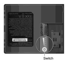
The value of the corresponding green segment indicates the relative percentage of the battery charge. The battery pack is fully discharged when you see no segment glowing green.
