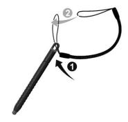
Insert the other loop end to the tether holder on the Tablet PC (as indicated by 1 below). Then, insert the stylus end through the loop (as indicated by below) and pull it tight.
