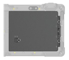
2. Lift the battery pack off the compartment.
