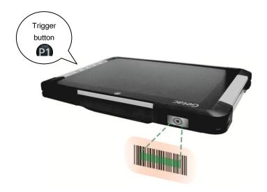
**NOTE:** If the code being scanned is highly reflective (e.g., laminated), it may be necessary to tilt the code  $+5^{\circ}$  to prevent unwanted reflection.
