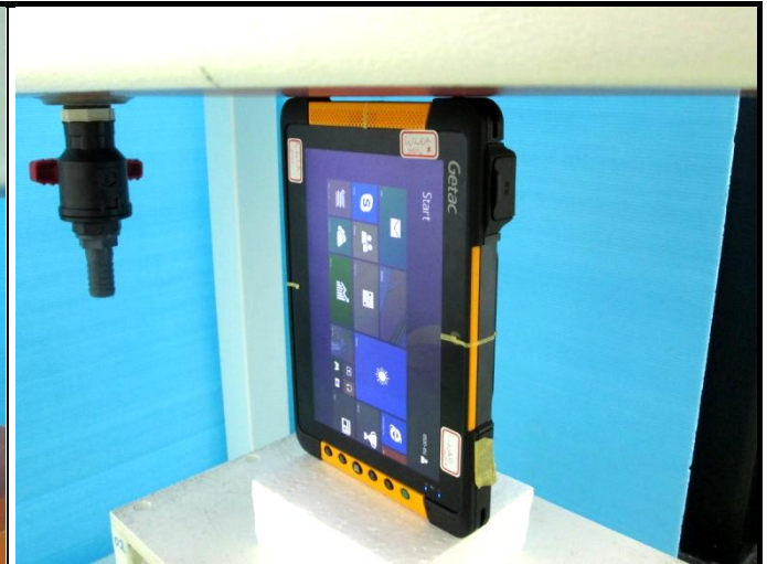
Left Side of EUT with 0 cm Gap (EUT Standalone)
