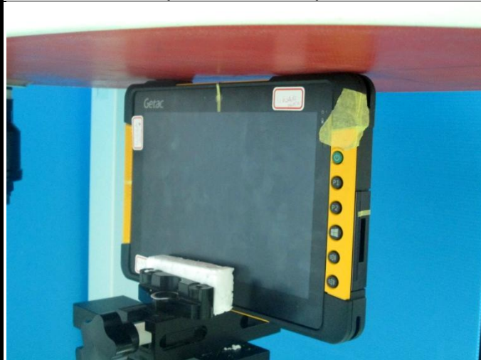
Top Side of EUT with 0 cm Gap (EUT Standalone)
