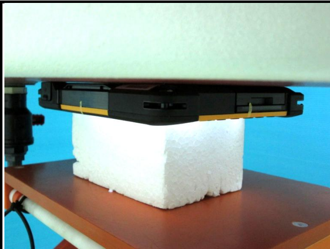
Rear Face of EUT with 0 cm Gap (EUT Standalone)
