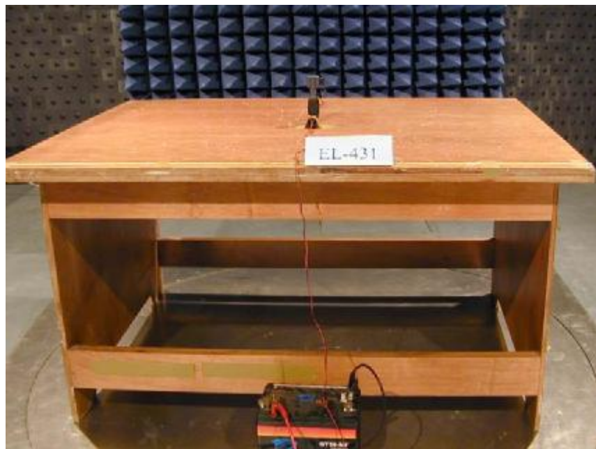
Photo 2: Radiated Emission Test Set-up
