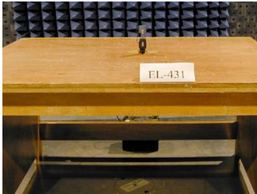
Photo 2: Radiated Emission Test Set-up
