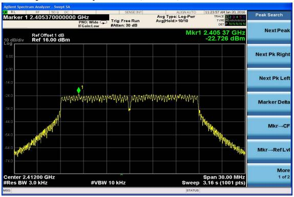
**Power Spectral Density Test Plot (CH-Mid)**
