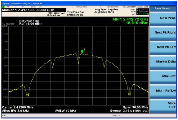
**Power Spectral Density Test Plot (CH-Mid)**
