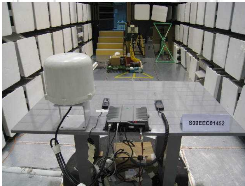
Protection of Aeronautical Radio Navigation Satellite Service Test Setup (Rear View)
