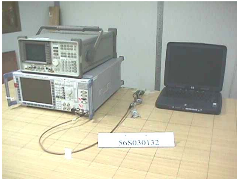
Carrier Frequency Separation Measurement Test Setup
