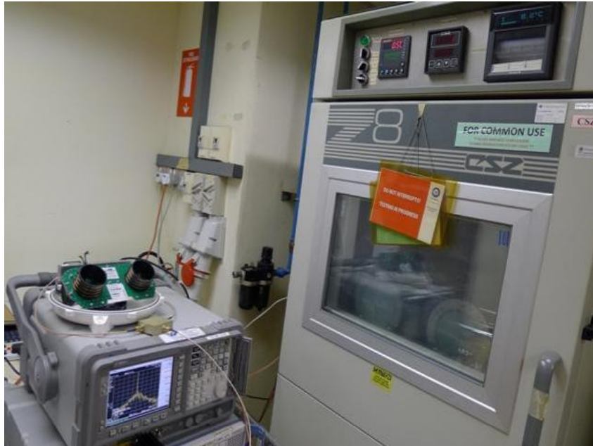
Frequency Stability (Voltage Variation) Test Setup
