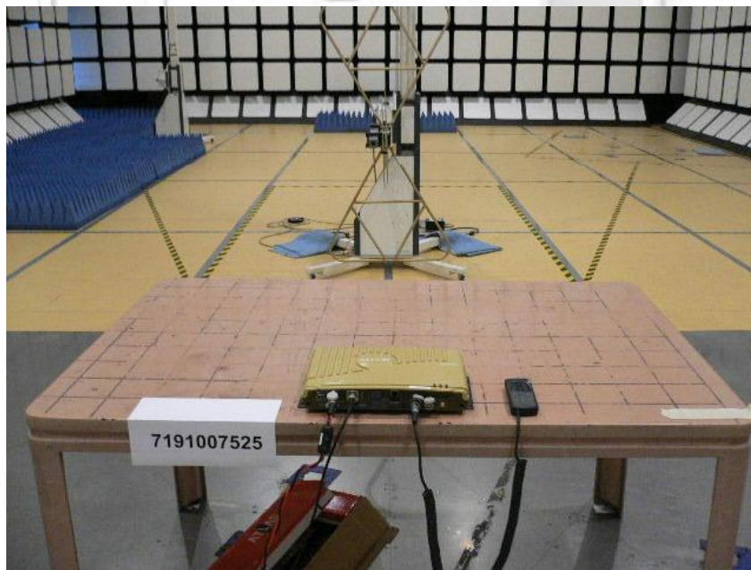
Radiated Emissions Test Setup (Rear View)
