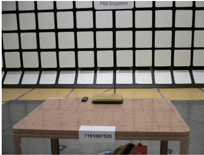
Radiated Emissions Test Setup (Front View)
